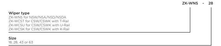
Note on ordering: Every kit contains a pair of wipers. Two wipers per slider are always required.
