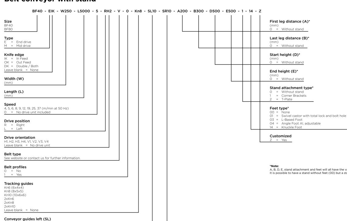
A, B, D, E, stand attachment and feet will all have the value 0 if the conveyor is defined without a stand. It is possible to have a stand without feet (00) but a stand attachment must be selected.
