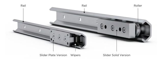
Rollco C-Rail compact and quiet linear guide with low friction. The system is suitable for applications in dusty environments where precision is not the main factor. It is a simple and cost-effective linear bearing. The stainless steel version is perfect for applications where corrosion resistance is important.
