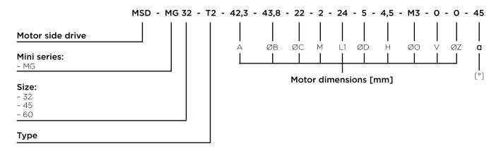
Dimension ØO is also used for tapped holes. In case of tapped holes, prefix M must be applied.
