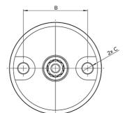
Adjustable Feet, Base 80 with anti-slip/vibration plate and fixing holes Die-cast zinc with a black powder coat
