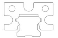
\* MF contact surfaces are tolerance match to the guiderail to ensure perfect sealing
